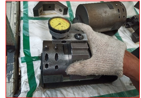
Master setting with dial gauge
